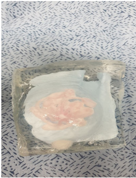
Figure 2. Made by mixing the colorant / contrast agent (barium) with silicone
