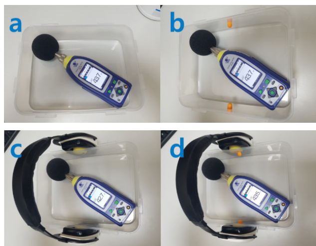
Figure 2. Measuring method (a) General MRI noise (b) Earplugs (c) Headset (d) Earplugs + Headset
