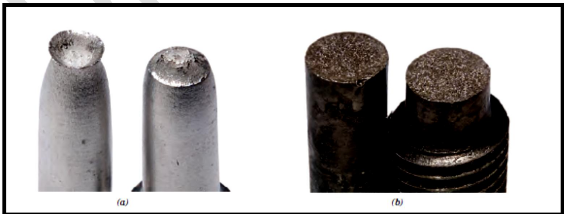
Figure(3.3): (a) Cup-and-cone fracture in aluminum. (b) Brittle fracture in a mild steel.
