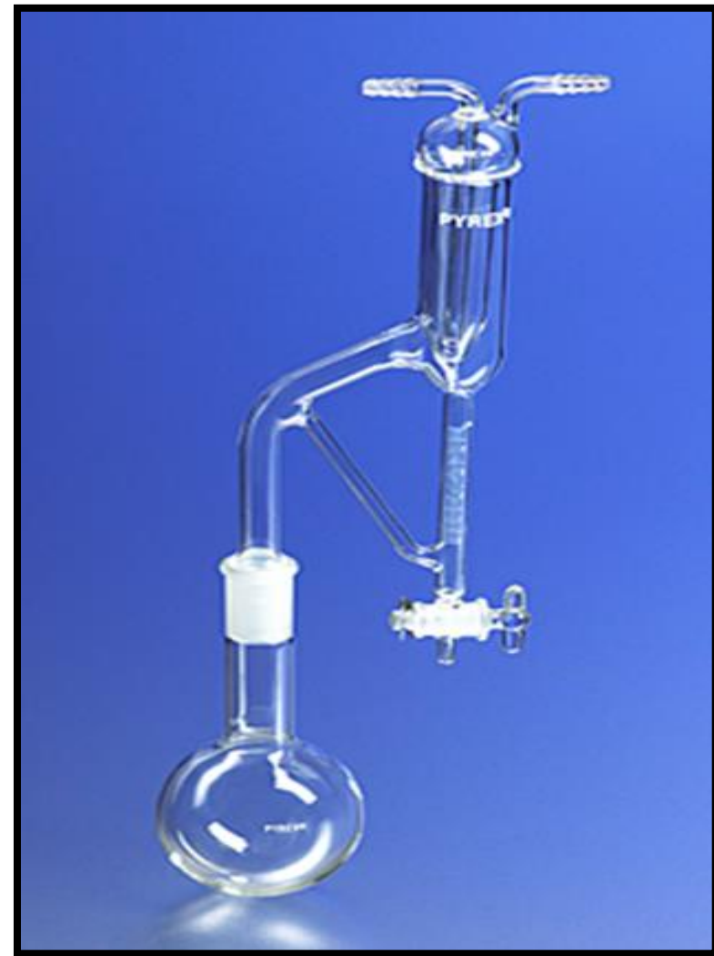
Clevenger (Oil lighter than water)
