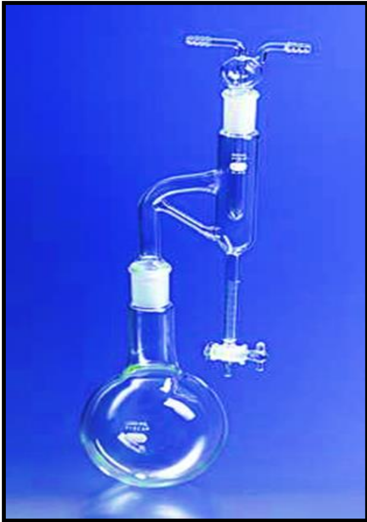
Clevenger (Oil heavier than Water)
