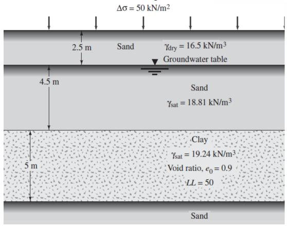
A soil profile is shown. Laboratory consolidation tests were conducted on a specimen collected from the middle of the clay layer. The field consolidation curve interpolated from the laboratory test results as shown. Calculate the settlement in the field caused by primary consolidation for a surcharge of 60 kN/m<sup>2</sup> applied at the ground surface.
