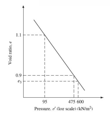
Two points on a curve for normally consolidated clay have the following two points on a curve for normally consolidated clay have the following
