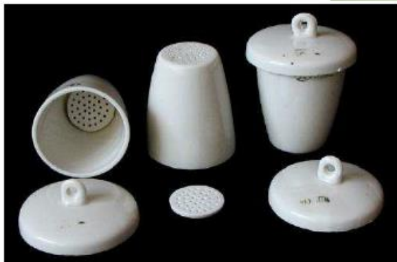
Porcelain crucible (Ignition up to 1000 °C)
