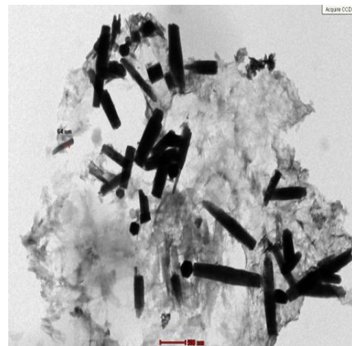
Figure 6: TEM images of ZnO Rod shaped fused at centre to form a radiating structure as observed in SEM
