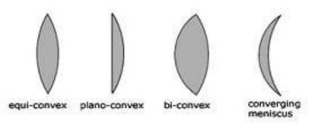
All four types of convex lens are converging lenses. That is, they bring parallel rays of light to a focus, producing a real image.
