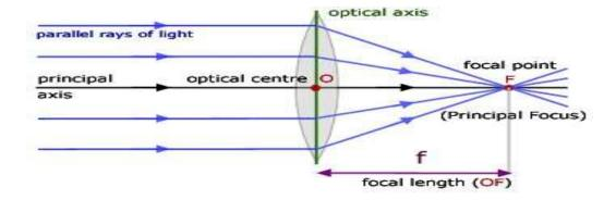
The basic ray diagram for a convex lens introduces a number of important terms
