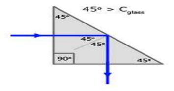
For 90° deviation, a 90° isosceles glass prism is used. In this way the incident ray and the reflected rays are normal to the surfaces they enter and leave(and therefore unhindered). Total internal reflection occurs on the hypotenuse
