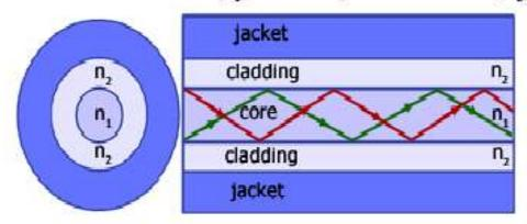
Optical fiber has a number of advantages over copper wire:
