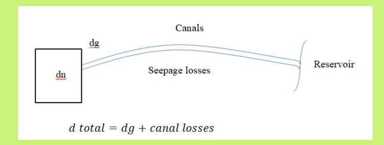
**Conveyance efficiency:** Is the percentage ratio between the gross depth of water to the total irrigation depth.
