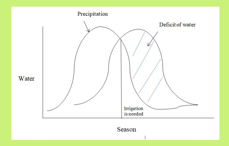
Net depth of irrigation  $(d_n)$ : Is the depth of water applied and stored in the root zone  $(d_n)$  it is the only water available for plant growth.
