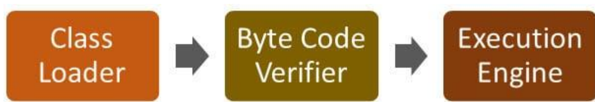
Working of Java Virtual Machine (JVM)
