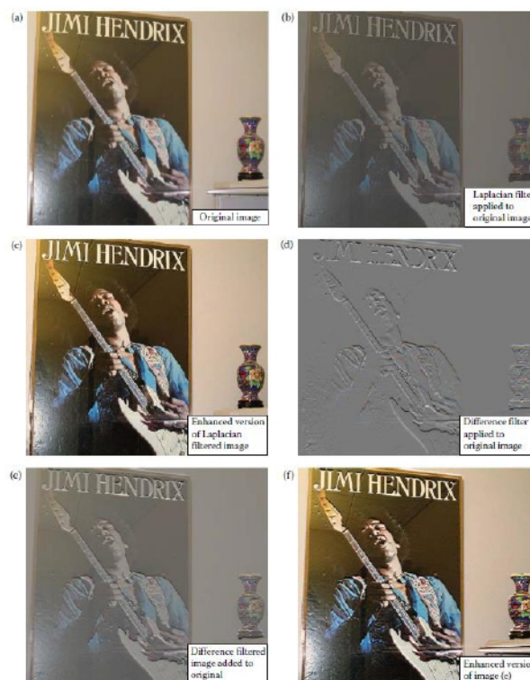
Figure 53. Enhancement Filters. (a) Original image, (b) image after Laplacian filter, (c) contrast enhanced version of Laplacian filtered image, compare with (a) and note the improvement in fine detail information, (d) result of a difference (emboss) filter applied to image (a), (e) difference filtered image added to the original, (f) contrast enhanced version of image (e).
