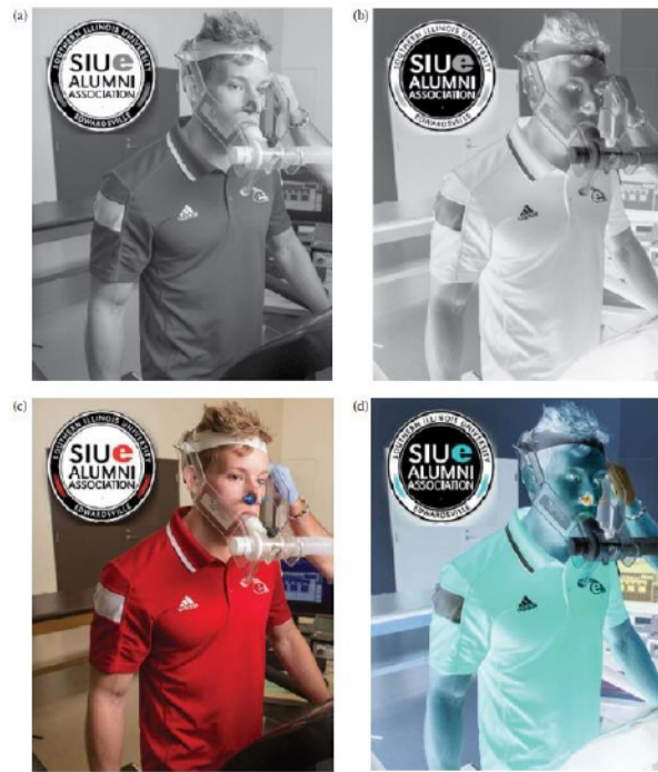
Figure 50. Complement Image- NOT Operation. (a) monochrome image, (b) NOT operator applied, (c) color image, and (d) NOT operator applied
