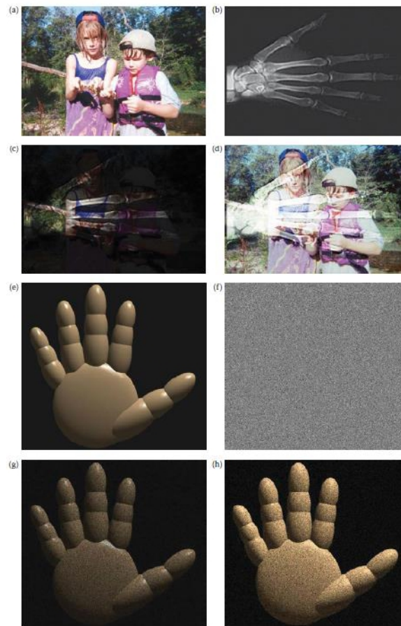
Figure 48. Image Multiplication. (a) original image, (b) x-ray image of a hand, (c) images (a) and (b) multiplied together which superimposes the hand onto the original, (d) the output image (c) after image enhancement, (e) a computer generated image of a hand, (f) Gaussian noise image, (g) the result of multiplying image (d) and image (e), this operation adds texture to a computer generated image, and (h) image enhanced version of the hand image with texture added by multiplication.
