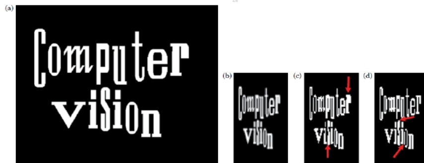
Figure 32. Spatial Reduction. (a) Original 512×512 image, (b) spatial reduction to 64×128 via averaging, (c) spatial reduction to 64×128 via median method, note the space in the “s” and “r” is filled in, and (d) spatial reduction to 64×128 via decimation method, note the “o” is split and “s” is filled in.
