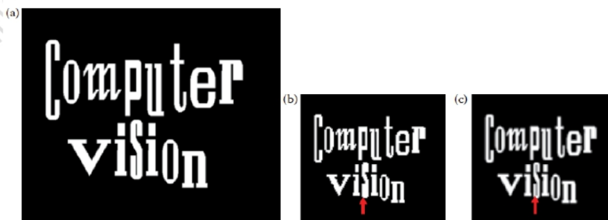
Figure 33. Decimation and Anti-aliasing Filter. (a) Original 512×512 image, (b) result of spatial reduction to 128×128 via decimation, and (c) result of spatial reduction to 128×128 via decimation, but the image was first preprocessed by a 4×4 averaging filter, an anti-aliasing filter. Note that the “s” is still clear and the “o” is not so jagged.
