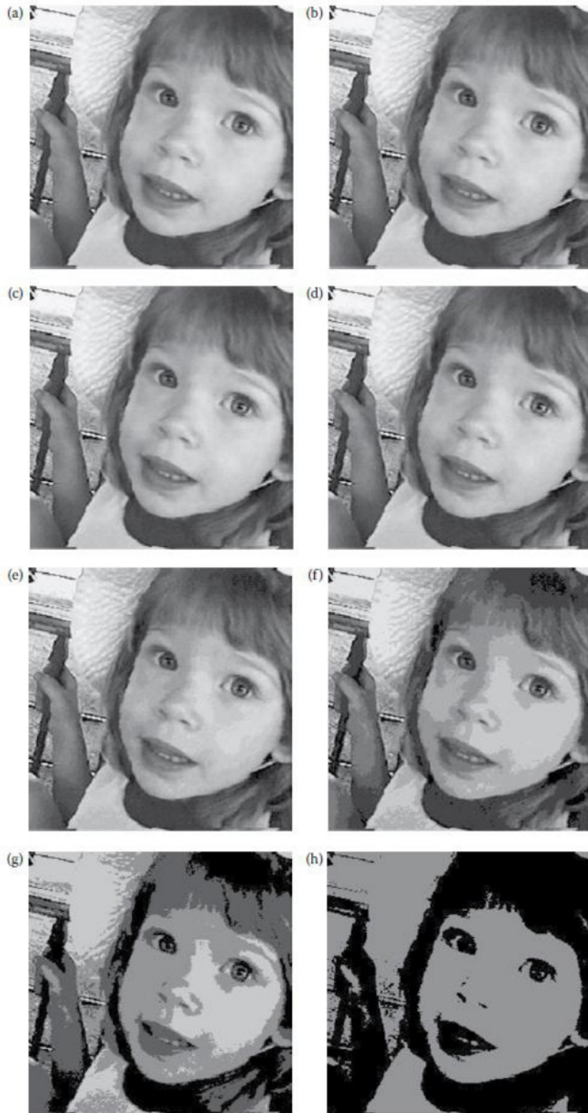
Figure 30. False Contouring. (a) Original 8-bit image, 256 gray levels, (b) quantized to 7 bits, 128 gray levels, (c) quantized to 6 bits, 64 gray levels, (d) quantized to 5 bits, 32 gray levels, (e) quantized to 4 bits, 16 gray levels, (f) quantized to 3 bits, 8 gray levels, (g) quantized to 2 bits, 4 gray levels, and (h) quantized to 1 bit, 2 gray levels.
