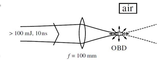
In the generated plasma, optical phase conjugation can occur and thus the laser source can be damaged by the back-scattered light, especially if
