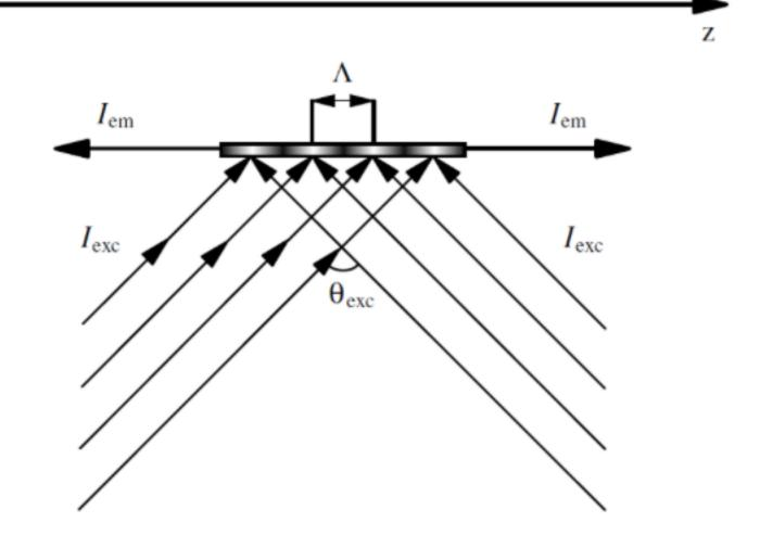
Because of the interference of the laser light along the z axis in the sample only a certain wavelength  $\lambda DFBL$  can be amplified. The gain period is determined by the angle  $\theta exc$  between the two pump beams and their wavelength  $\lambda exc$ :
