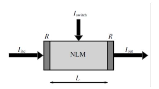
The operation of this device is better the higher the quotient (1-T)/(1-R). Besides nonlinear absorption the nonlinear Kerr effect can also be applied for optical bistability. If the Kerr material is used as the nonlinear material, the nonlinear transmission of the device can be written as
