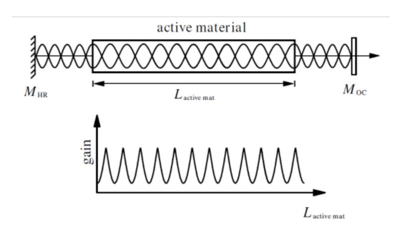
The standing wave occurs in the laser resonator as a result of the steadystate field condition with nodes of the electric field at the mirror surfaces.
