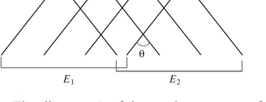
The distance  $\Lambda$  of the grating structure follows from the angle  $\theta$  between the beams and the wavelength  $\lambda$ exc of the pump light as:
