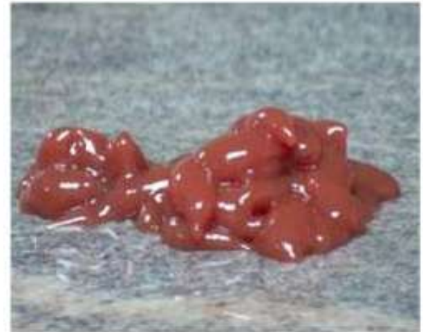
Once the vibration stops, the ketchup returns to its original viscous state.
