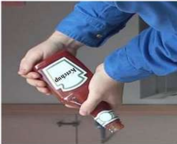
Ketchup is a good example of a thixotropic substance. It does not flow even when the bottle is held upside down.
