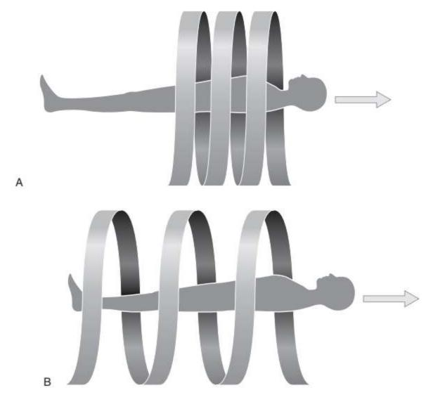
(A) Pitch is low. The table moves less for each tube revolution. The image is sharper.
