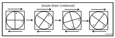
For non-coaxial deformations, the orientations of the principal strain axes are different for different amounts of strain, while for coaxial deformations they always point in the same directions (same orientation, different lengths).
