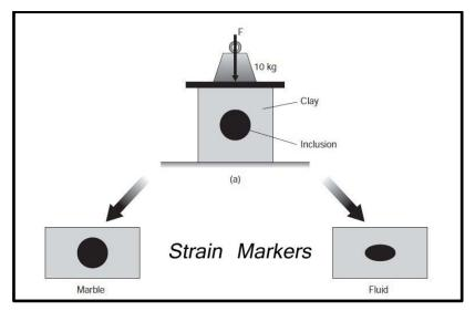
**Passive strain markers**: <u>are elements in the body that have no mechanical contrast or</u> <u>differences; they deform in a manner indistinguishable (unclear) to that of the whole</u> body.
