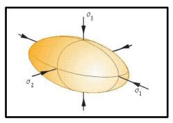
*Strain ellipsoid (deformation ellipsoid)*: Are the three dimensional figure enclosing three perpendicular strain axes which are:
