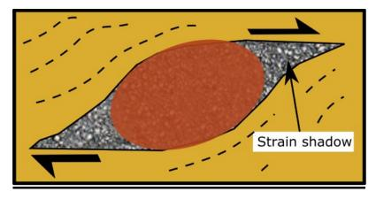
We place a marble within a cube of clay, and as we load the block it deforms into a rectangular box. After sectioning, the marble remains undistorted! So, using the marble as the basis for strain analysis we conclude there is zero percent strain (or X/Y = 1), yet looking at the clay you clearly see that strain has accumulated. In fact, we determine a strain ratio, X/Y, of 1.8 for the clay.
