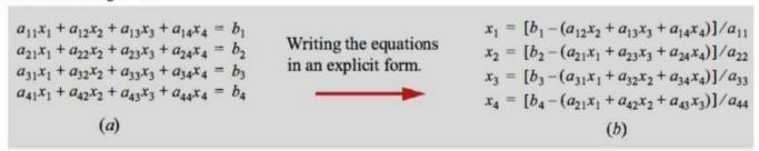
Figure 3-13: Standard (a) and explicit (b) forms of a system of four equations.
