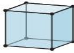
Primitive cubic lattice
