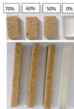
Figure 2. Shows a photograph of wood-plastic composite samples.
