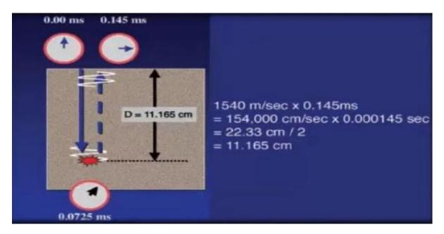
If an ultrasound pulse is transmitted into the body and time until echo returns is measured, it is simple to calculate the depth of the interface that generated the echo, provided the propagation velocity of sound for the tissue is known.
