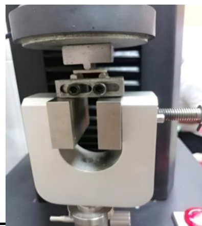
Figure 3 - Specimens in the universal testing machine (a) unloaded and (b) loaded conditions.
