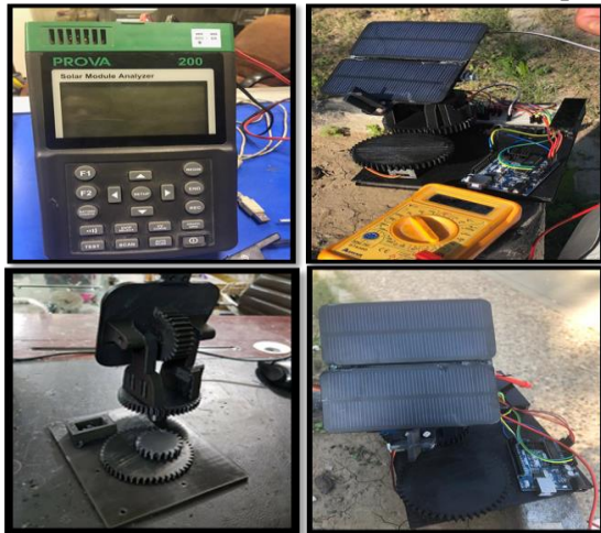
Figure 6. Mechanical arrangement of the tracking system
