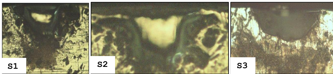
Figure 4. Penetration of fusion zone with different energies S1, S2 and S3.
