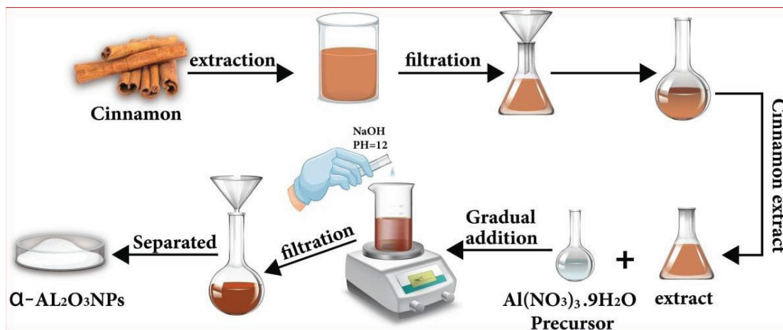
FIGURE 2. The preparation steps of \alpha -Al 2 O 3 Nps powder using Cinnamon extract.
