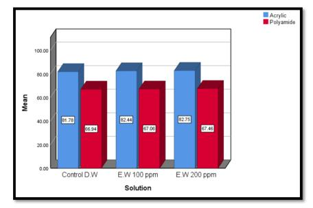
Results of the one-way ANOVA of the hardness test demonstrated no statistical difference between the groups, as shown in Figure 1.
