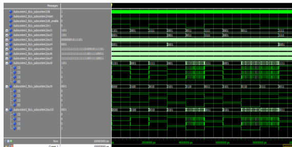
Fig.12. The details of 8QAM band pass modulated signal.
