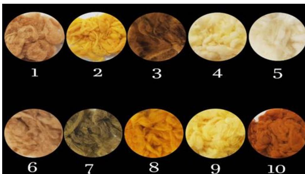
Figure 12. Shapes of cotton fibers dyeing to Schiff base and complexes. 1-H 2 Ldfm, 2-[Mn(LdfmL)(Phen)], 3-[Co(Ldfm)(Phen)], 4-[Fe(Ldfm)(Phen)]Cl, 5- [Ni(Ldfm)(Phen)]6-[Cu(Ldfm)(Phen)],7-K[Ag(Ldfm)(Phen)],8- [Cd(Ldfm)(Phen)], 9- [Hg(Ldfm) (Phen)], 10-[Pb(Ldfm)(Phen)].
