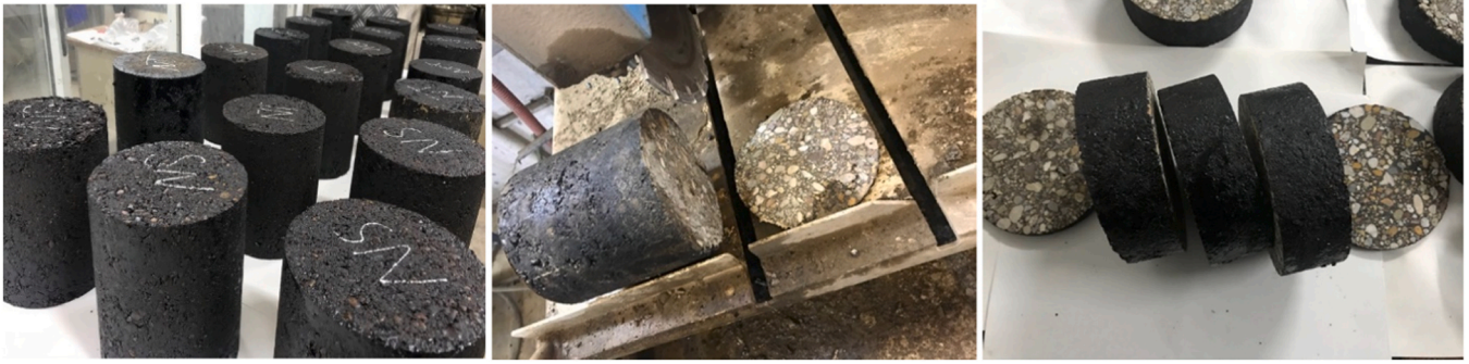
Fig. 5. SGC compacted samples and cutting.
