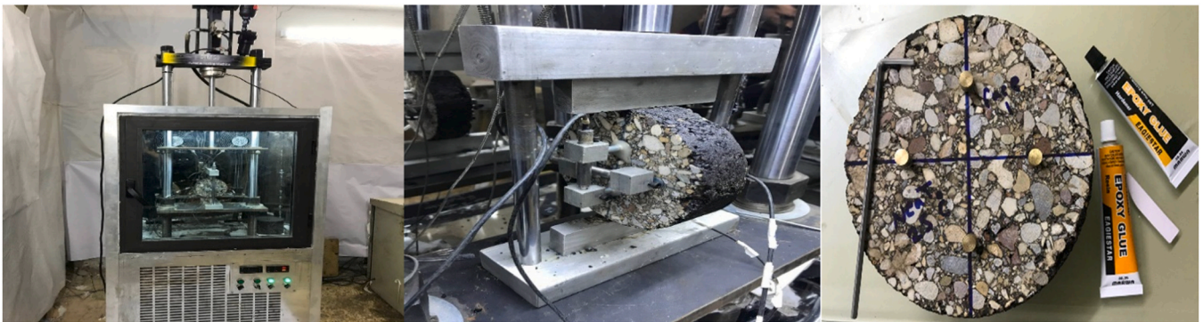
Fig. 6. Preparing IDT test specimen for testing.
