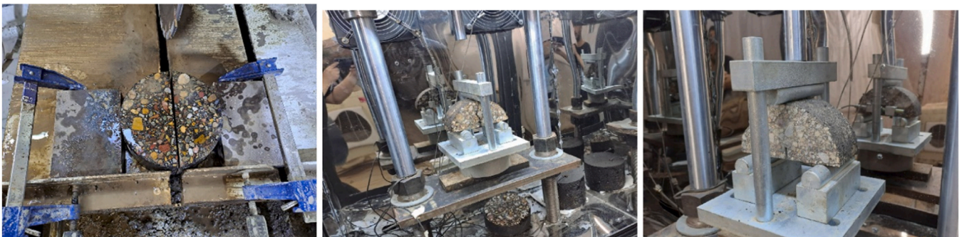
Fig. 7. Testing configuration for the SCB.
