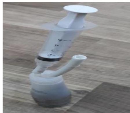
Figure 3.Hydrogen gas drying and storage system
