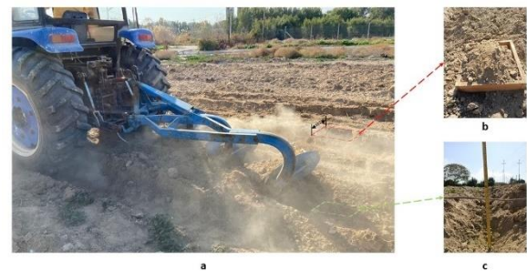
Fig. 2 Field experiment a. Mechanical unit b. Wooden frame c. Depth measuring tape. Source: created by the authors
