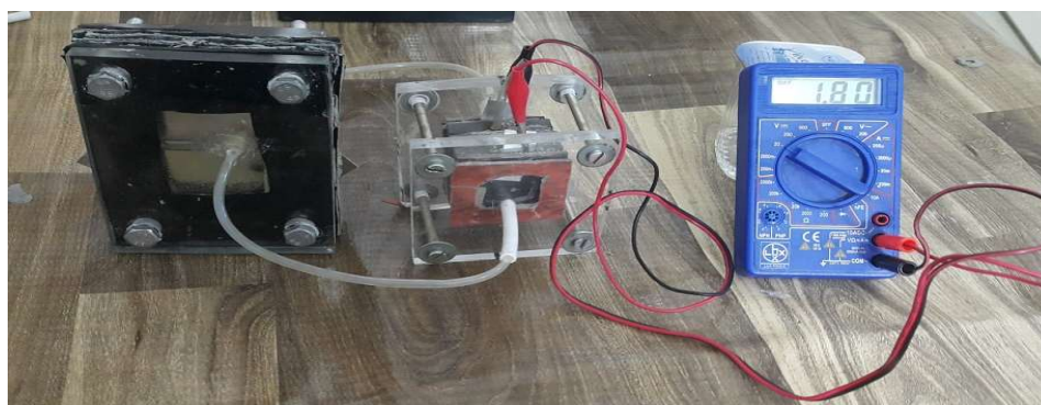
Figure 7. An alkaline fuel cell of electricity production.
