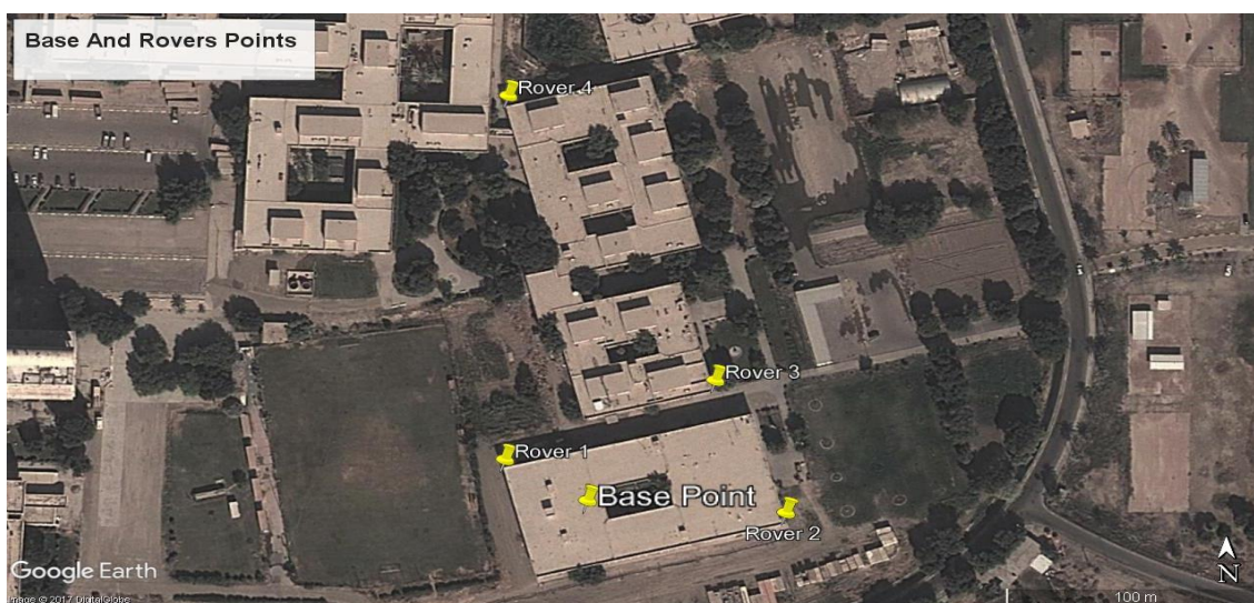
Figure 5- a Satellite Image for Base & Rover Points Locations
