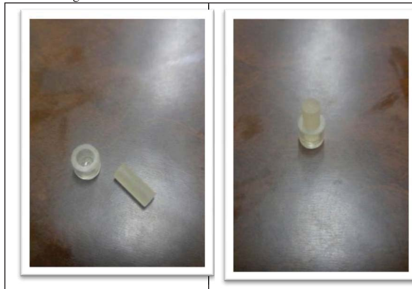
FIGURE 2. The crucible made of Pyrex and the epoxy rod, for thermal expansion coefficients measurements of bitumen samples.
