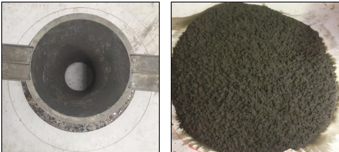
Figure 2. Slump Flow test.
