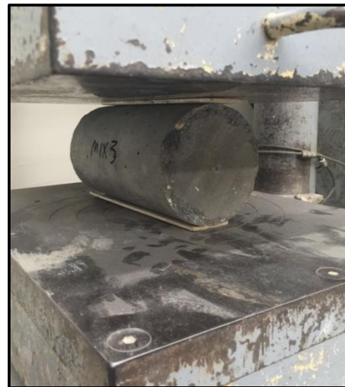
Figure 5. Splitting tensile strength test.
