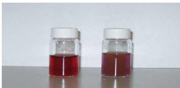
Fig. 2 The G NPs which is prepared by chemical reduction method in global lab (Bahadory , 2008).
