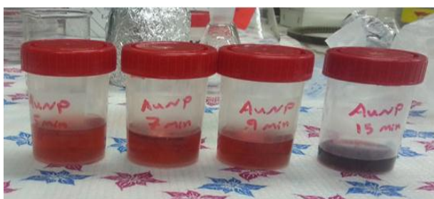
Fig. 1 The Gold Nanoparticles which is prepared by chemical reduction method by variation the reduction time from adding point.
