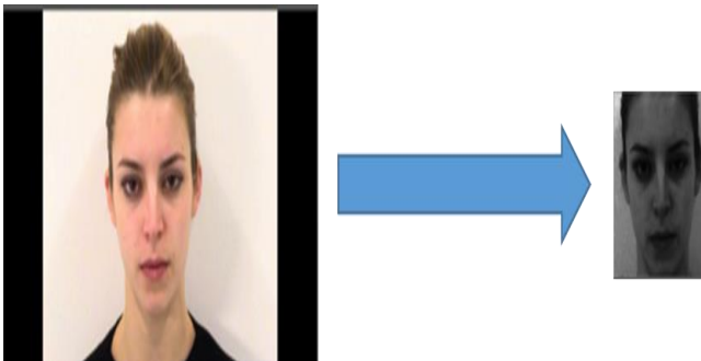
Fig. 7. Example of an original video image and how it will be after applying the preprocessing face detection and postprocessing steps.
