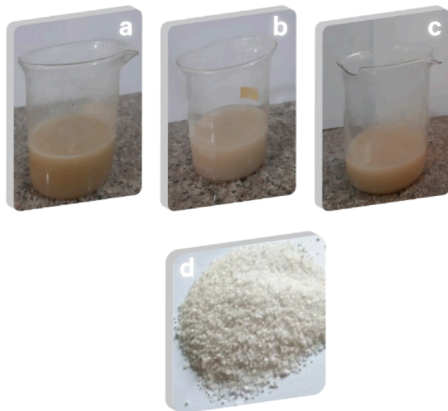
Fig. 2. Colour change of solutions of Al 2 (SO 4 ) 3 and bio-reductor of Boswellia carterii resin extract (a) dark Peggy, (b) Milky, (c) Pale Peggy, and (d) \gamma -Al 2 O 3 –NPs powder.
