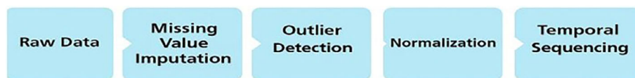
Figure 1. This schematic summarizes the preprocessing steps applied before model training: raw data collection, missing value imputation, outlier removal, normalization, train-test splitting, and temporal sequencing for time-series forecasting.
