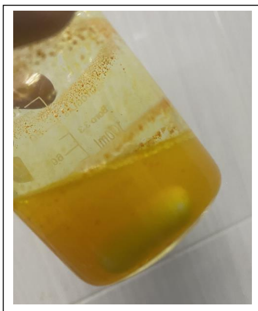
Fig 2: Example on failed CRN formulae using HPMC as stabilizer.
