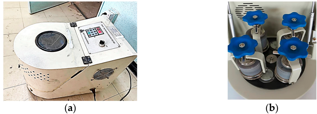
Figure 2. (a) Rotating bench-top automatic ball-milling machine used to blend the powders and (b) metal containers or jars in which the powders were placed.
