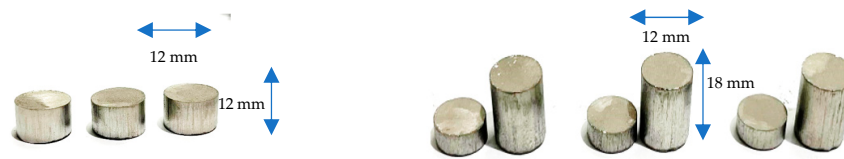
Figure 4. Green compact samples after compaction.
