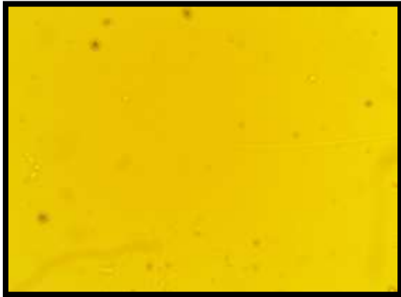
FIGURE 2. Tracks of alpha particles emitted by (Rn-222) seen in (CR-39) detector.
