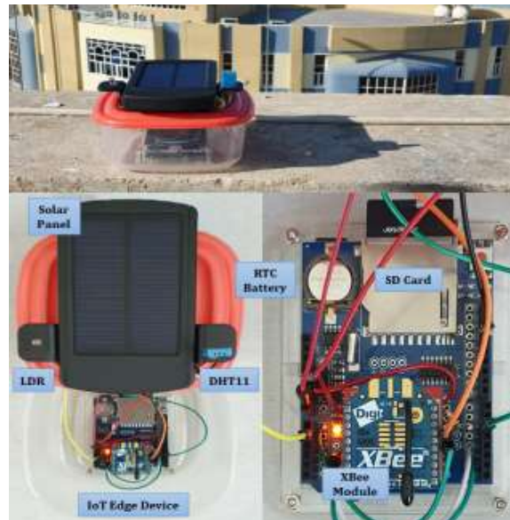
Fig. 3: Developed IoT edge device with PV module
