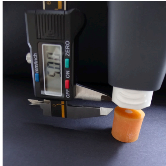
Fig. 1. Non-thermal plasma device (PiezoBrush® PZ3 Handheld Device, Relyon Plasma, Regensburg, Germany) was fixed at a distance of 5 mm from specimen.
