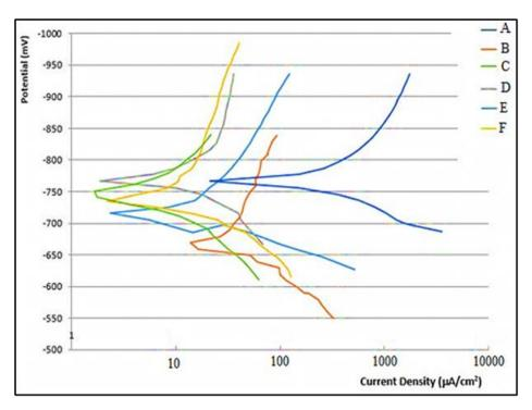
Figure 4: Polarization curves for specimens AA2024-T3 in 3.5% NaCl media.
