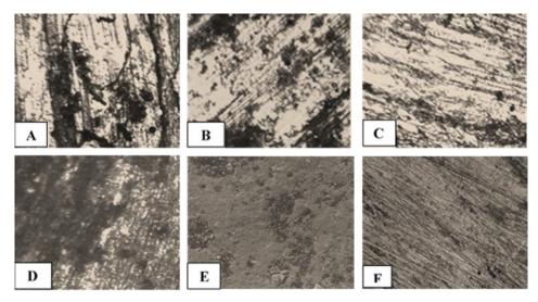
Figure 5. Micrographs indicating the pitting corrosion for all specimens of Al- Alloy 2024-T3 after corrosion test in sea water solution at 100 X.
