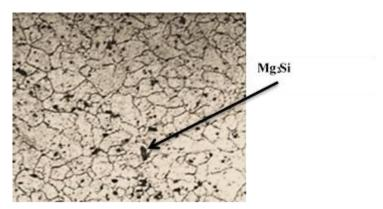
Figure 3. The microstructure of base metal AA 2024-T3, 500X
