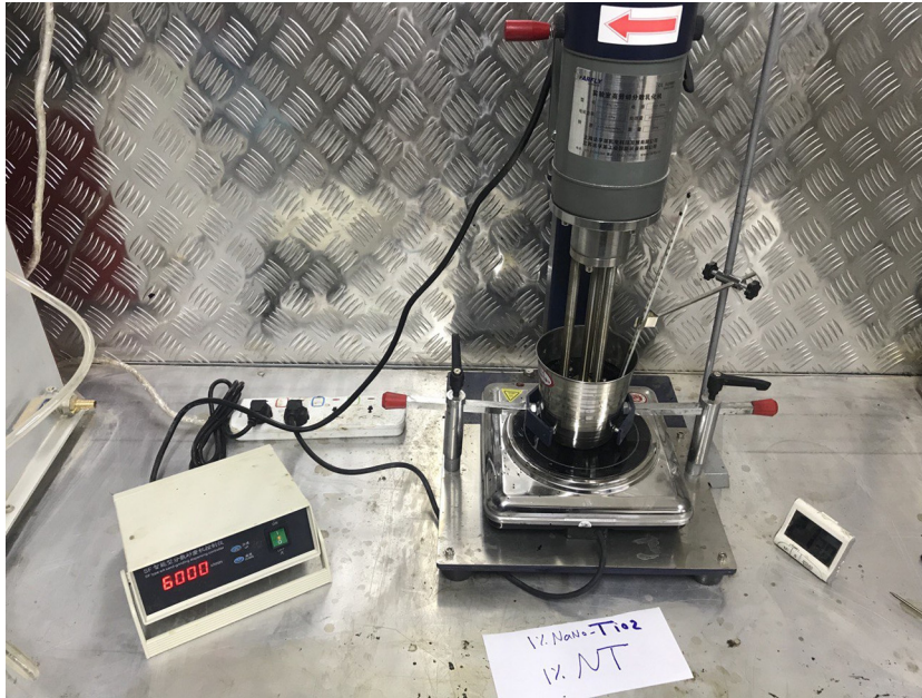
Figure 3: Mixing of nanomaterial with asphalt.
