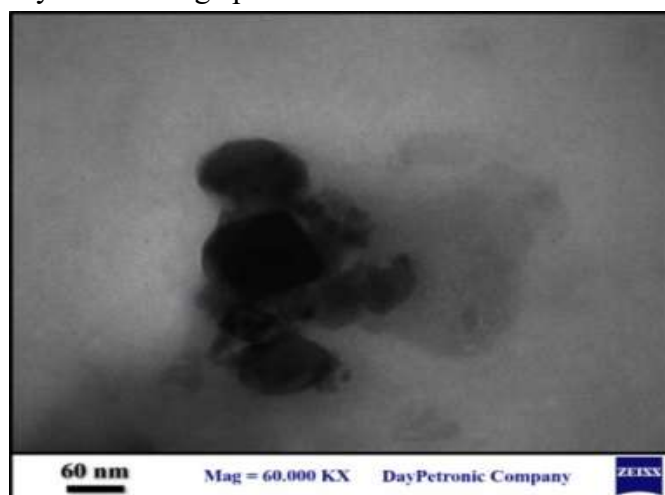
Figure 7. TEM for \alpha -Fe 2 O 3 NPs powder within 60 nm
