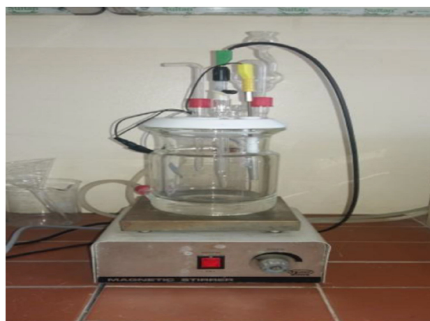
Fig. 2. The corrosion cell.
