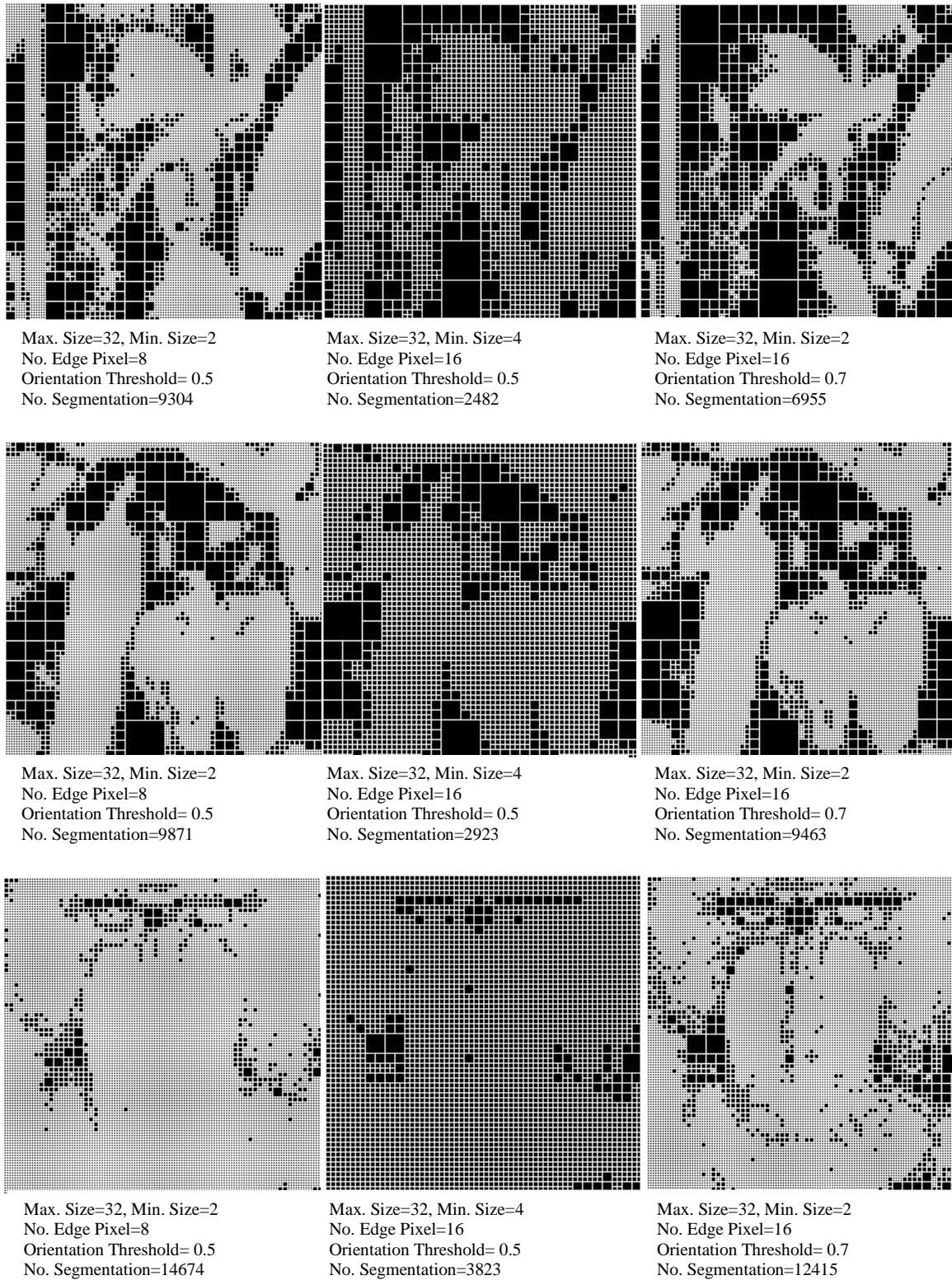
Fig 3: Examples of segmented tested images with different partitioning control parameter values.
