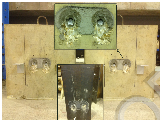
Fig. 17. Slab spalling after push-out Test 6
